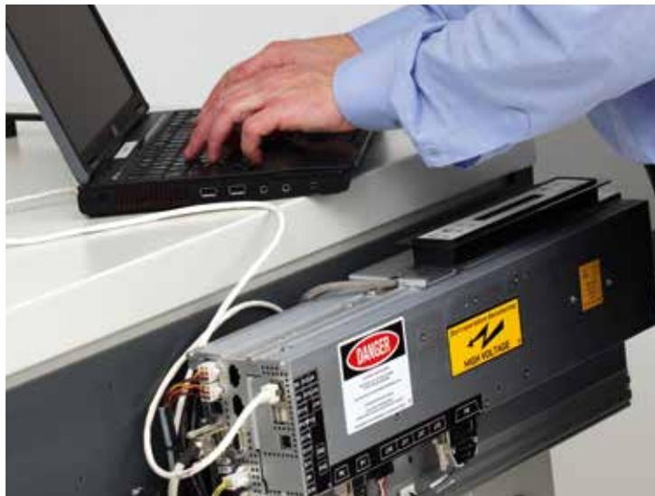
Glunz & Jensen's Remote Enabling System is included as standard and is used to configure the processor and allow for convenient remote service access via the internet.
