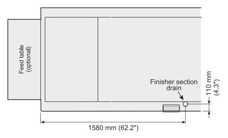
Prepare the installation site for drain connection according to the illustration. Please also refer to the "Space requirements" on page 12.
