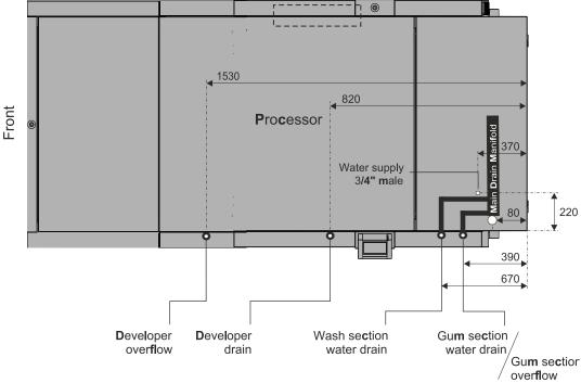
Prepare the installation site for water supply and drain connections according to the illustration. Please also refer to the "Space requirements" on page 12.
