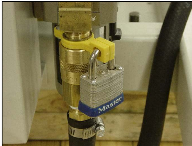
Figure 17. SLEEVE VALVE IN DOWN POSITION AND LOCKED.
