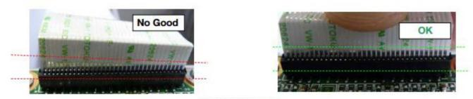
Head error 1A39: The drive circuit in the head can be damaged due to slant connection/terminals of the FFCs.
