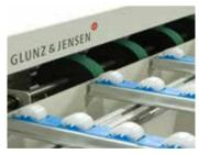
Optional Bridge Conveyor sections connect CtPs, processors and other conveyors to the CM62.
