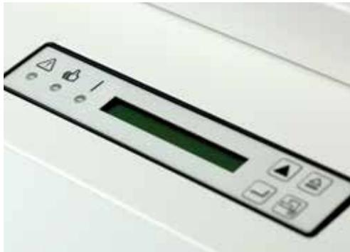
Gecko+ has a simple control panel with status/error information and function keys to quickly select between the four user-defined programs.
