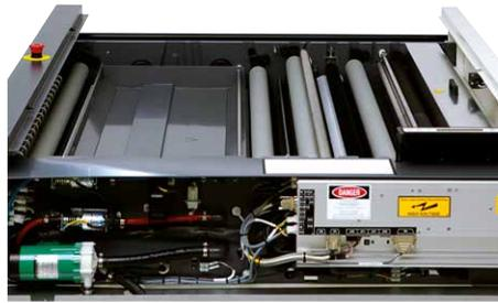
All electronics and mechanical components are located on the sides of the processor, for easy and convenient access during maintenance.
