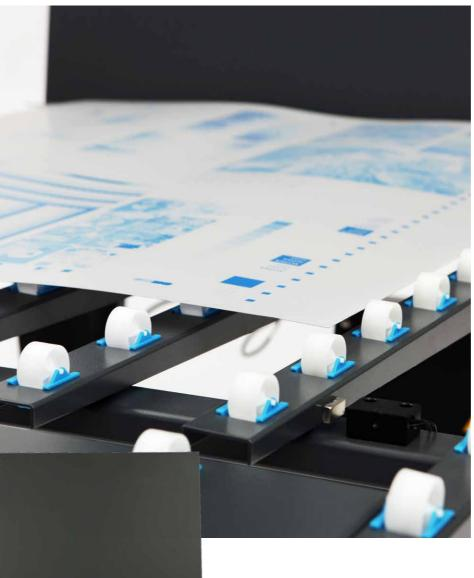
The trolley separates from the PRO Stacker, enabling the stack of plates to be conveniently moved to the press or to storage. The PRO Stacker's conventional stacker design features a belt driven conveyer to transport the plate from the processor to the trolley.
