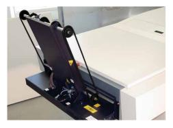
The System Conveyor can conveniently hinge onto the processor or stand alone. Both configurations can be flipped up to give access to the setter.
