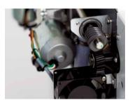
The COU+ uses a reliable and maintenance-free worm gear drive system to drive rollers and brushes.
