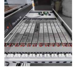
Easy pull-out access for convenient maintenance of electronic balasts and lamps in the main exposure and light finisher sections.
