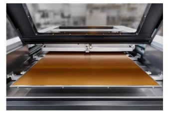
The processor includes a self-adhesive panel which securly holds the plate in place, without the need for punching holes.
