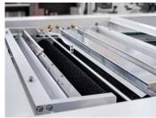
The **processor** section includes integrated heating and cooling device for solvent temperature control and automatic replenishment.
