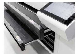
Consistent exposure quality is achieved by precise control of all relevant processing parameters such as lamp temperature, UV exposure time, temperature of exposure surface, UV output etc.
