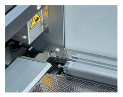
The updated pin bar loading system has fewer moving mechanical parts, which minimises the risk of plate infeed problems and improves serviceability.
